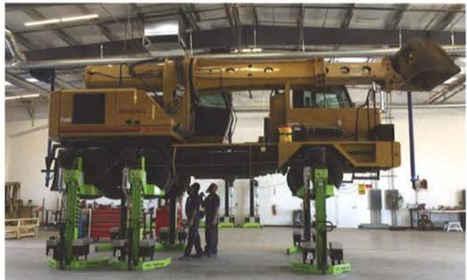
Merced Irrigation District – A new portable lift system was installed in the vehicle maintenance shop to prevent mechanics from kneeling down or bending over in awkward postures for prolonged periods.
